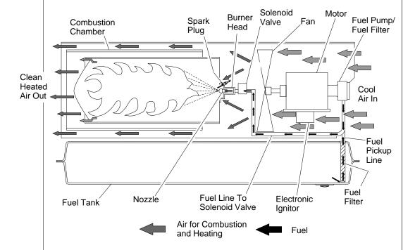
Figure 3 - Cross Section Operational View
